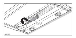
Note for dismantling the cooker hood: Undoing the screws on the left and right inside the housing releases the spring mounts, allowing the appliance to be removed from the unit.
